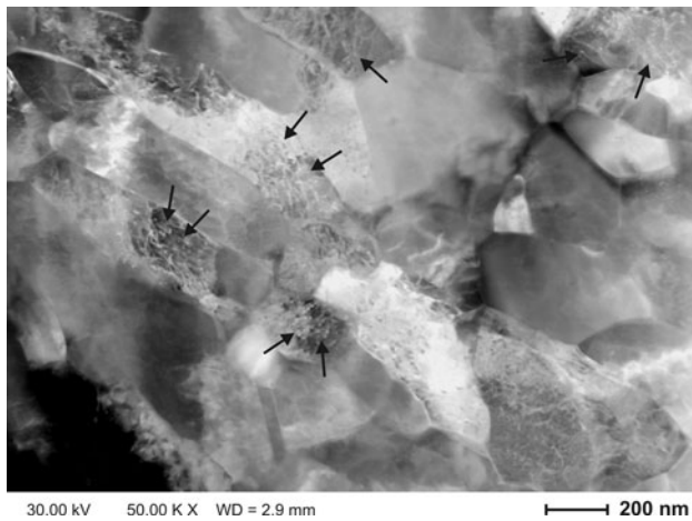
Fig. 7 STEM micrograph of UFG 6060-T6, E8 with homogenous ultrafine slightly elongated grains in dark field contrast (small arrows point to dislocations)
